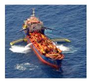
The Aktea OSRV is an oil tanker built in 1989 and contracted by EMSA to cover the Aegean Sea area. Transporting oil is the main commercial activity of the vessel. The Aktea OSRV has a storage capacity for recovered oil of 3 000m<sup>3</sup>, a heating capacity of 3 000kW and a pumping capacity of 1 000m<sup>3</sup>/h.
